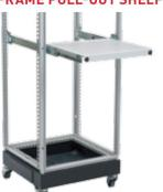
Frame Pull-Out Shelf allows easy access to shelf-mounted devices. The shelf is 16 gauge steel with 12 gauge steel supports. The entire assembly is finished with RAL 7035 textured gray polyester powder paint. The shelf mounts to the front and rear frame uprights. Load rating is 110 lb. (50 kg).
